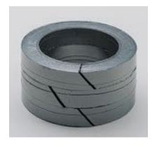
5300 (GTPI) Die-Formed Inhibited Graphite Rings Chesterton 5300 is a self-lubricating, low friction, high purity, precompressed, die-formed ring manufactured from pure graphite ribbon tape without any fillers binders or resins. Each ring is engineered to produce an accurate specific density for compression resistance, elasticity and retention of size and shape, all of which are necessary to provide the best possible valve sealing performance.
